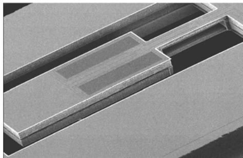
Piezoelectric films on a micro-mechanical system to control the deflection of a cantilever
